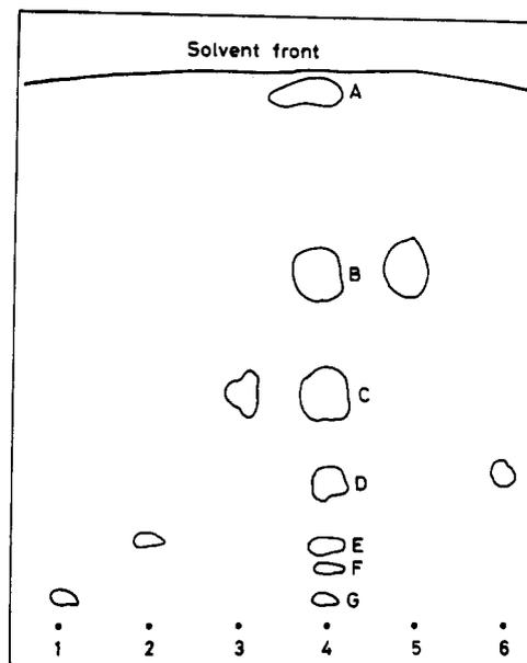
Figure 2. Separation of components of free lipids of wound periderm by thin-layer chromatography. 1, monoplaminin; 2, dipalmitin; 3, oleic acid; 4, free lipid fraction of wound periderm; 5, tripalmitin; 6, lauryl alcohol. A, hydrocarbon; B, triglycerides; C, free fatty acids; D, fatty alcohols; E, diglycerides; F, unidentified; G, monoglycerides. Experimental details are outlined in the text.
