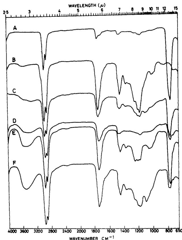
**Figure 4.** Infrared spectra of various components of aliphatic fraction of suberin. A-F refer to the components isolated by TLC as shown in Figure 3. Components D-F show strong absorption at 2.85  $\mu\text{m}$ , indicating the presence of hydroxy groups.
